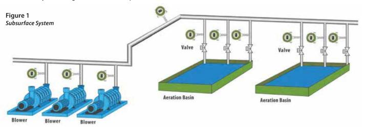
A successful aeration control system is dependent upon the efficient operation of its system components. The components for each region may include an air flow valve, air flow meter and DO {dissolved oxygen} meter. The valve, commonly a butterfly valve, is usually installed downstream of the flow meter. Much of aeration control is predictive, as there is a nonlinear relationship between the airflow and dissolved oxygen content which creates a lag time to reach equilibrium.
