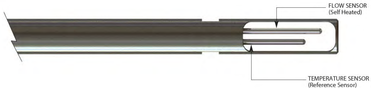
Figure 19 - One of the sensors is self-heated, and the other sensor measures the gas temperature.
