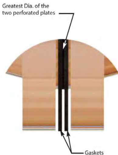
Figure 5 - Captive Flow Conditioners are designed to be separated by one pipe diameter.
