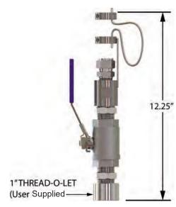
Note: User needs to weld a 1" female threadolet (of appropriate radius) to mate with existing pipe after a 1" hole has been drilled in pipe. The 1" Male Coupling of the Sage Isolation Valve Assembly will thread into the user's 1" threadolet.
