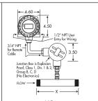
**SRP In-Line**<sup>4,6,7</sup> Flow Element is In-Line style consisting of a choice of 316 Stainless Steel Schedule 40 Flow Bodies sized from 1/4" x 6" long to 4" x 12" long
